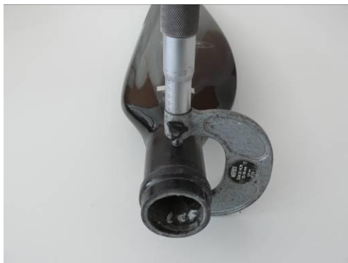
Diameter 45,00 mm (measured by micrometer)
