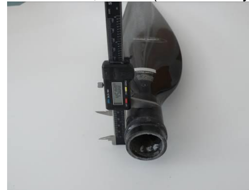
Diameter 45,00 mm (measured by slide calliper)
