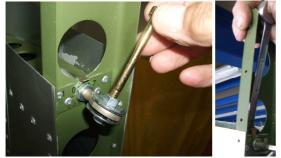
9. Pull out the hinge, self locking nut and tab washer
