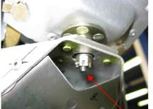
3. Use M8 nut wrench to release and unscrew castle nut from the rudder lower hinge.
