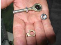
10. Set a new tab washer (size 8) onto the hinge thread. It is not recommended to straighten up and use original washer, due to possible cracking when being bent repeatedly.
