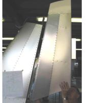
7. Use a slide calliper or another suitable rule to measure distance of the hinge eye rear edge from the fin rear spar and note this value.
