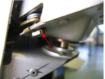
5. Use M9 nut wrench to unscrew both screws attaching the cables to the rudder and pull the cable ends slightly out and fix together by a wire, so that to not be drawn into the fuselage.
