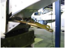
6. Lift the rudder up and remove from the fin.
