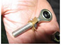
11. Set the hinge back on the fin spar, the washer must be on the outside of the spar as shown on the picture.
