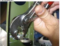
16. The washer bigger tab must be bent forward by a suitable tool (e.g. flat screwdriver and hammer) to protect the washer from rotation. The end of bigger tab should be pressed up to the self-locking nut edges.
