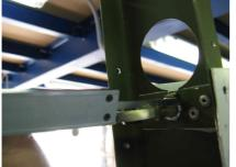
8. Screw M6 nut on a sufficiently long M6 bolt (80 mm), then put a washer (25 mm diam.) on the bolt and insert into the hinge from above. Put another washer on the bolt from below and tighten with another M6 nut. Now set M13 nut wrench through a lightening hole on the self locking nut inside the fin (right figure below) and turn the M6 bolt to release and unscrew the hinge.
