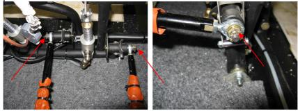
2. Use a suitable pliers to draw a cotter pin out of the castle nut securing rudder lower hinge.
