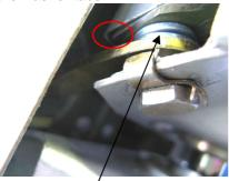
Note: The two ',normal" washers above the cable ends are installed to prevent cables from being chafed from the rudder front lower edge (marked red). Installation of these washers is recommended if not installed and there is an evidence of chafing in this area.
