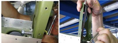
13. Measure the distance between hinge eye rear edge and fin spar and if different from the original one, then screw or release the hinge to adjust this distance.
