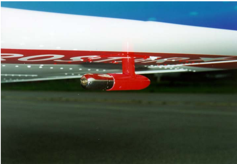
Fig. Pitot-static tube under the left wing
