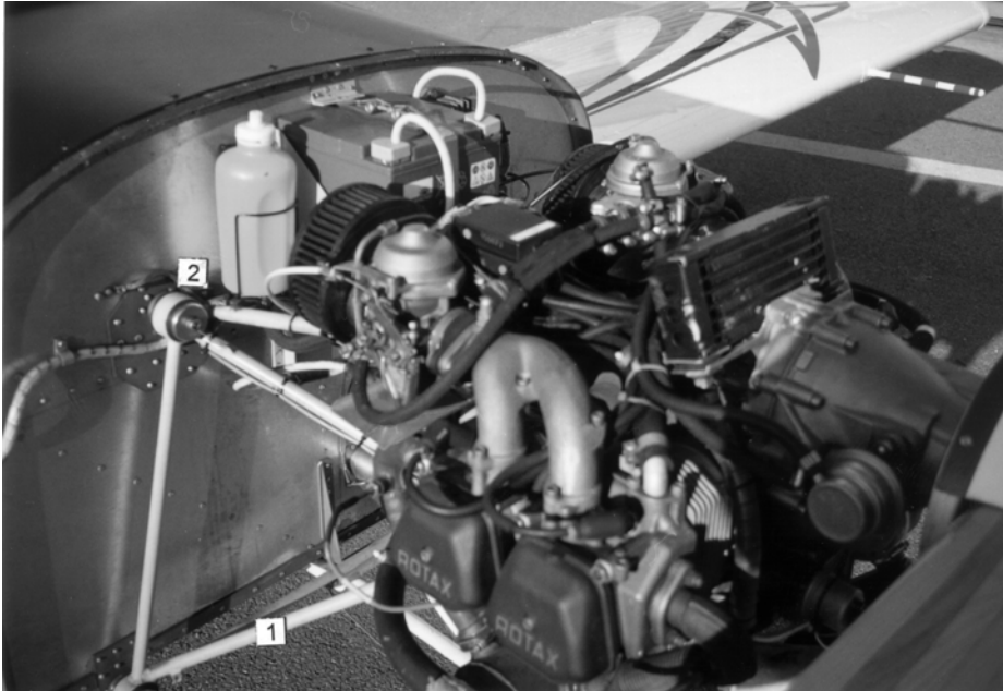
Fig. Engine mount 1- bed, 2 - rubber silentblock
