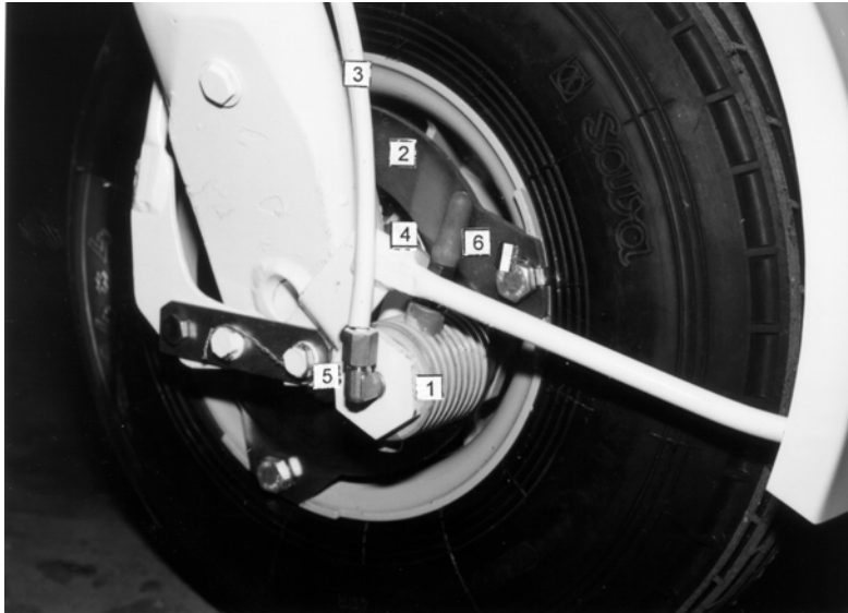
Fig. The brake on the left wheel 1 - brake caliper with the hydraulic cylinder, 2 - brake disc 3 - brake fluid hose, 4 - brake pad holder, 5 - terminal, 6 - air bleed screw
