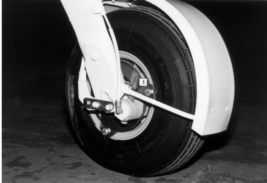
Fig. Brake system bleeding 1- Bleeding screw
