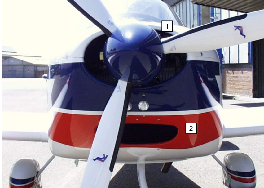
Fig. Rotax 912 engine cowlings 1 - upper cowling, 2 - lower cowling with cut-out for the radiator
