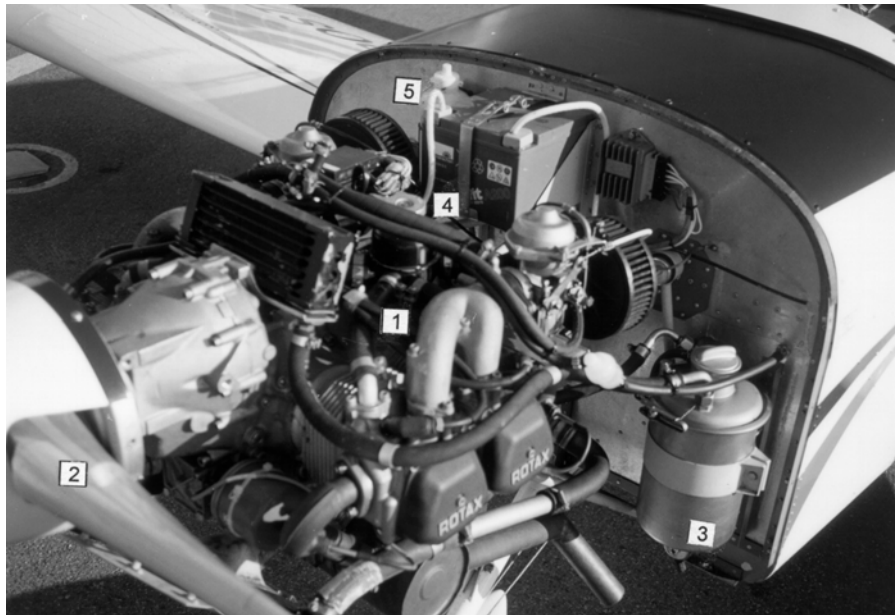
Fig. EV-97 Powerplant (standard powerplant) 1- ROTAX 912 engine (80 hp), 2 – V 230C prop, 3 - oil tank, 4 - coolant expansion tank, 5 - coolant overflow bottle
