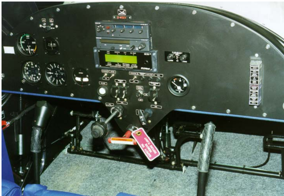
Fig.: Cockpit of the Ev-97 “EUROSTAR” model 2000 version R
