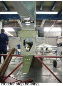
Rudder step bearing
