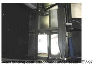
Check of rivet connections in the area of the main landing gear attachment
