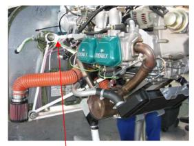
Nose landing gear leg area of hinges on the fire wall and at the engine (the critical place is indicated)
