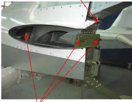
Stabilizer hinges Pin diameters: min Ø6-0.04 mm Ø8-0.05 mm
