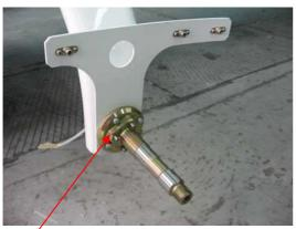
Attachment of the wheel axis with the nose landing gear leg
