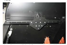
Attachment of the left upper engine hinge on the fire wall
