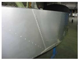
Area of the fuselage reinforcement Check of the hinge and riveted joints
