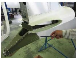
Towing equipment hinge Check of condition of rivet joints
