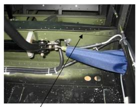
Area of connection of caps and webs (after drilling out of seats)
