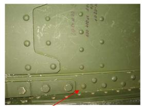
Area of bottom caps with wing-fuselage hinges
