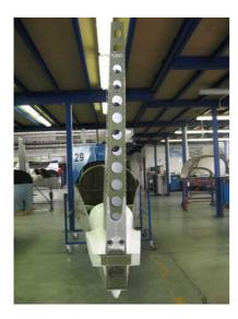
Fin spar with rudder hinges Check of spar caps (after dismantling of the rudder)
