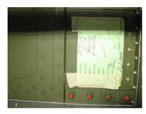
Bottom hinge Area of the wing spar (view against the flight direction, for information
