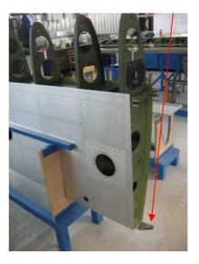
Rear hinge - max. Ø8+0.04 mm View on the bottom part of the wing in the area of wing-fuselage hinges (unfinished wing, only for info)
