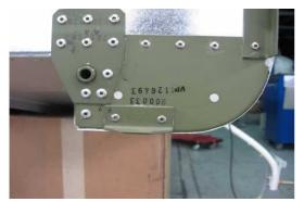
Left bottom engine hinge Check of the hinge and riveted joints (front view)
