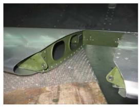
Stabilizer hinges Check of hinge rivet joints Hinges openings diameters: Ø8+0.04 mm; Ø6+0.03 mm
