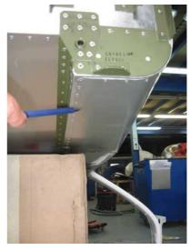
Bottom part of the fuselage under the left bottom engine hinge Check of the hinge and riveted joints
