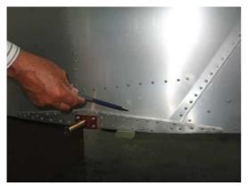
Area of the fuselage reinforcement Check of the hinge and riveted joints
